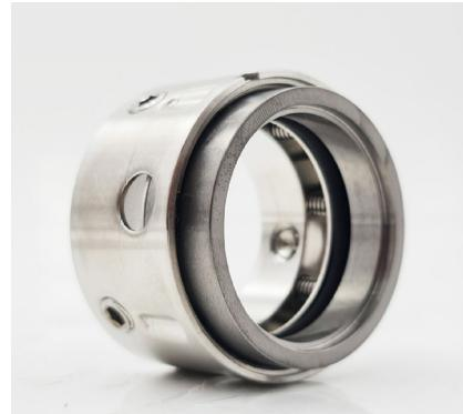
Pusher type rotating seal with PTFE wedge sealing on the shaft. This PTFE wedge retains the sealed fluid and follows the seal movement to compensate for shaft run-out and end play. This extremely effective seal designed to meet API standard and featuring multiple spring action, is suitable for a wide range of applications, particularly in refineries and petrochemical process plants. It is available in both metric EN 12756-L1K and imperial (inch) sizes.
